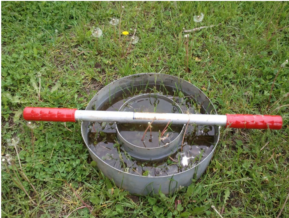
Photo 2: Example of infiltration progressing during field test.
