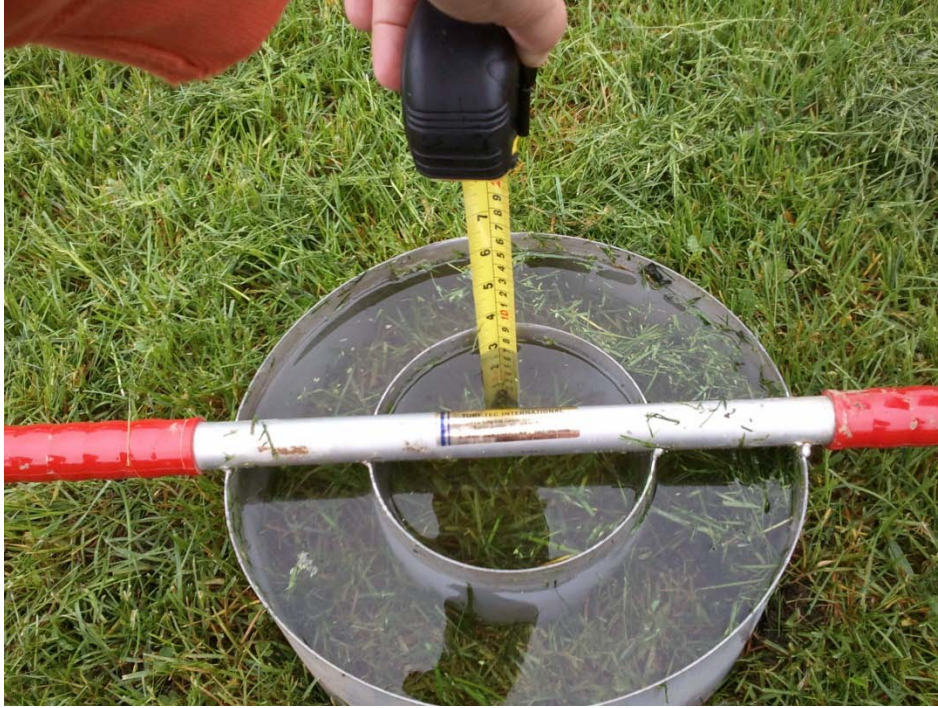
Photo 1: Double Ring Infiltrometer during the beginning of a field infiltration test.
