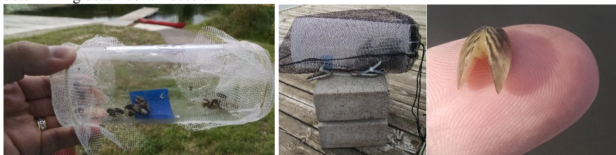
Acrylic tubes with fine mesh on each end. Zebra Mussel cages. Dead gaping zebra mussel.
