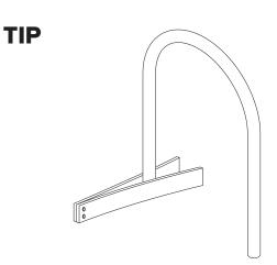
An easy way to brace the rack while the grout sets is to bolt two 1x4" boards together at one end and clamp them onto the legs of the rack like a clothes pin.
