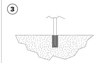
Place rack into holes, making sure the rack is level until the grout has set. 33"-36" of the rack should remain above the surface.
