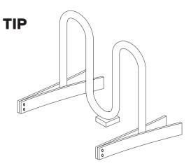
An easy way to brace the rack while the grout sets is to bolt two 1x4" boards together at one end and clamp them onto the rack like a clothes pin.
