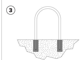
Place rack into holes, making sure the rack is level until the grout has set. 33"-36" of the rack should remain above the surface.
