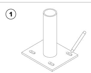
Place the rack in the desired location. Use a marker or pencil to outline the holes of the flange onto the base material.
