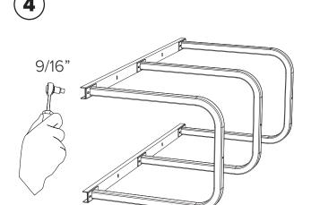
Once nuts are on, tip assembled rack over and use a 9/16" socket to tighten nuts. Before fully tightening nuts, make sure the racks are straight on beams. If using tamper resistant nuts, use access tool to tighten nuts. Do not overtighten the tamper resistant nuts. Tip rack upright.
