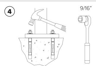
Thread nuts onto anchors, leaving approximately 1/4" of the anchor protruding, and tap into surface. Tighten nuts down to secure rack.
