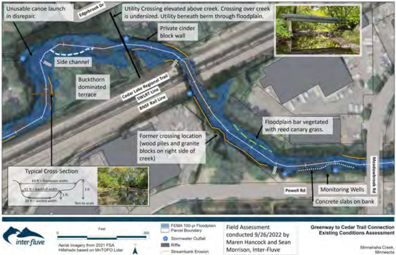
Figure 1: Existing conditions of the assessed reach.
