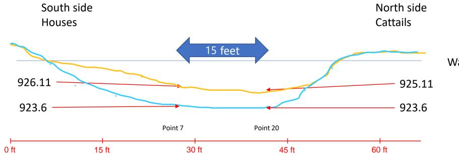
Dredge out the water way to a depth of 923.6 feet leaving a 3:1 slope towards the cattails to the north and a less severe slope to the south towards the houses. With in boat parking structures sediment to be removed to 924.6 at the waterway side sloping up towards the shore gradually to allow boats access. Along outside of docks a depth of 924.6 slowing down to main channel, and up towards shore.
