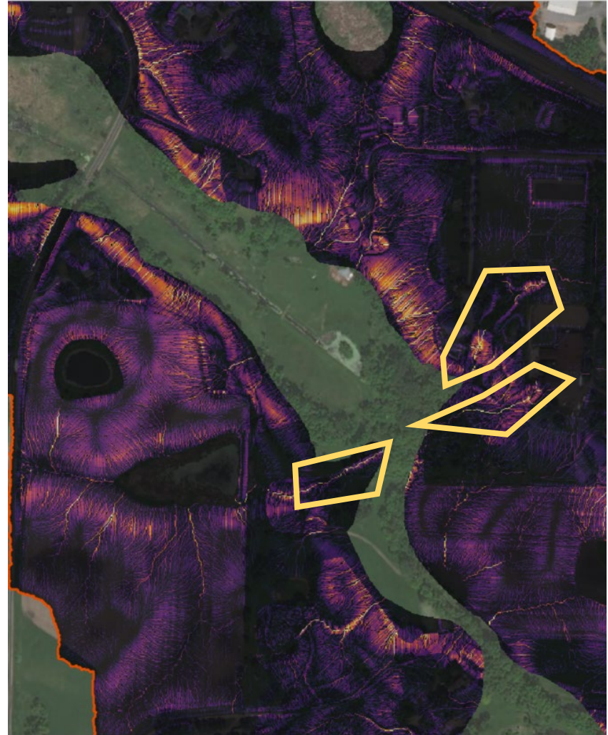
Figure 3-8 Current aerial photos of the areas downstream of Willow Rd. with erosion that has been field verified (left) and aerial photos with the USLE output overlay (right). Yellow polygons have been added to identify the areas of erosion.
