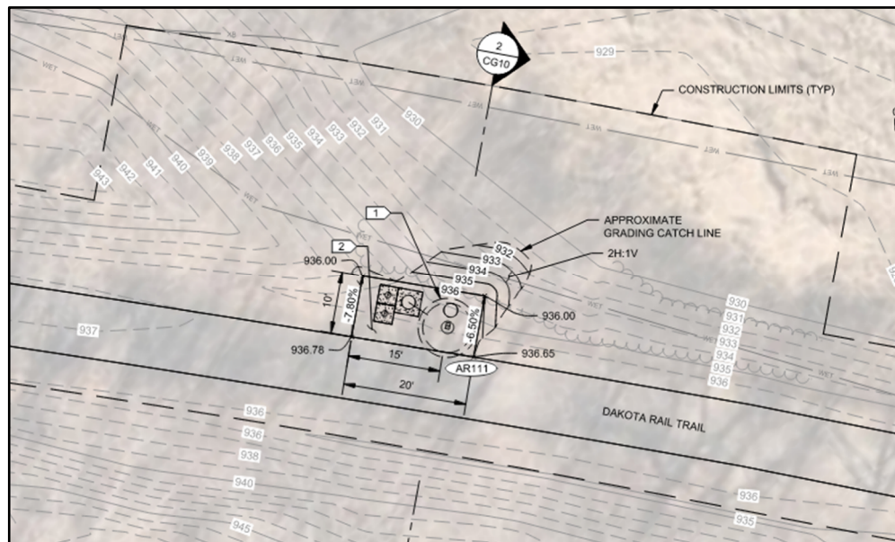
Figure 13 – AR111 Air Release Valve Location
