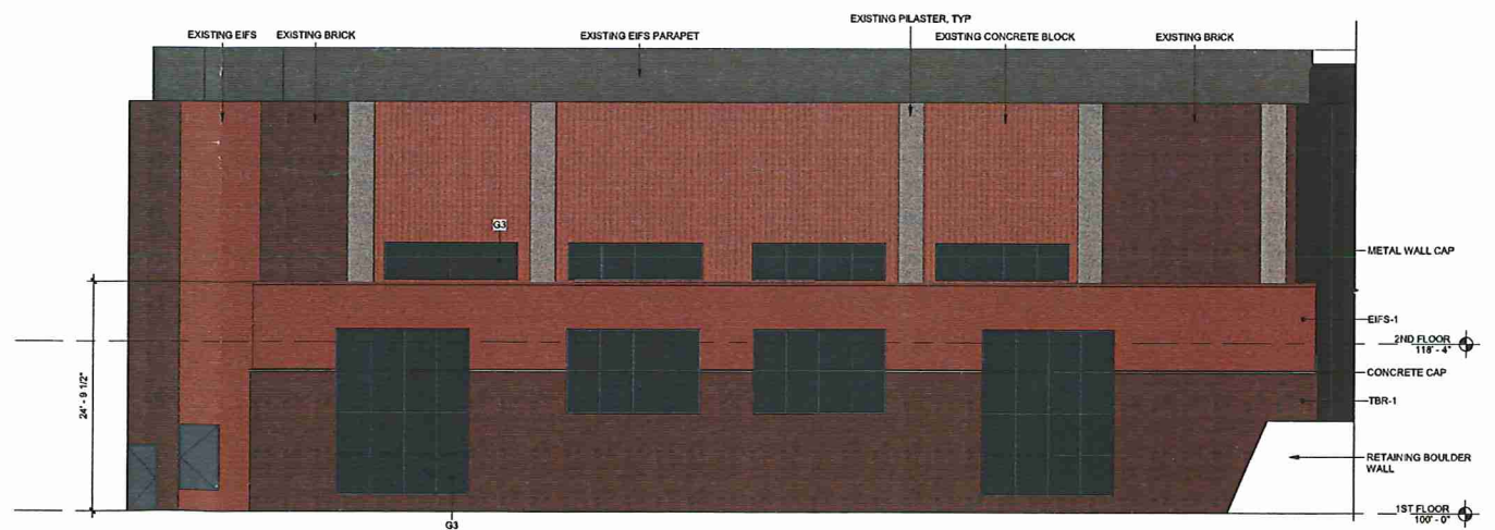
1 EXTERIOR ELEVATION - SOUTH 1/8" = 1'-0"
