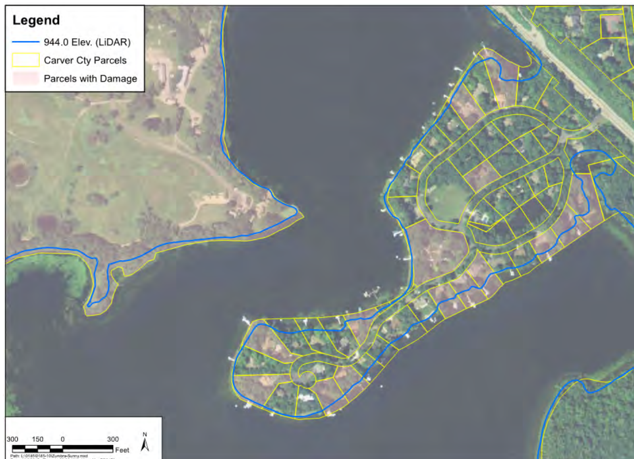
Figure 5. Flood damaged parcels and the 944.0 contour elevation (LiDAR). See Appendix E, Figure 2 for a more detailed breakdown of the parcel damage.
