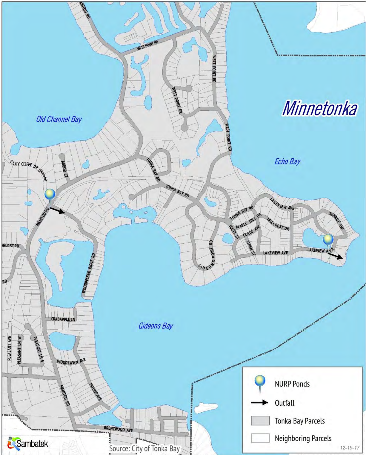
Figure 23 Existing Stormwater Ponds and Stormwater Outfalls
