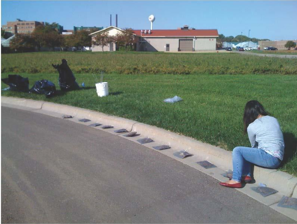
Figure 22. Installation of litterbags along a curb.
