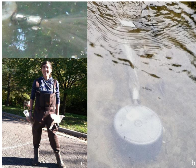
Figure 8. Seepage meters used to measure fluxes into or out of the streambed. (a) Close-up of hose-fittings used to attach the seepage meter to a plastic bag in which the change in volume of water over a set period of time is known. The valve is closed with the bag is removed or attached to avoid losing water. (b) Seepage meter deployed in streambed. (c) Measuring the volume of water in seepage meter bags 24 hours after deployment.
