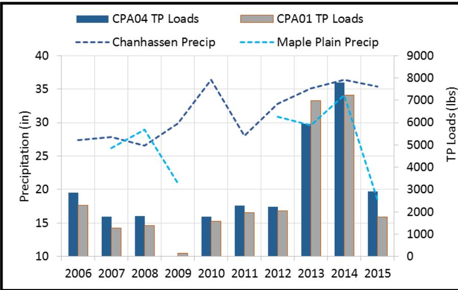
Figure 49. Comparison of annual precipitation and phosphorus loading at Painter Creek Marsh outlet (CPA04) and West Branch Rd (CPA01).
