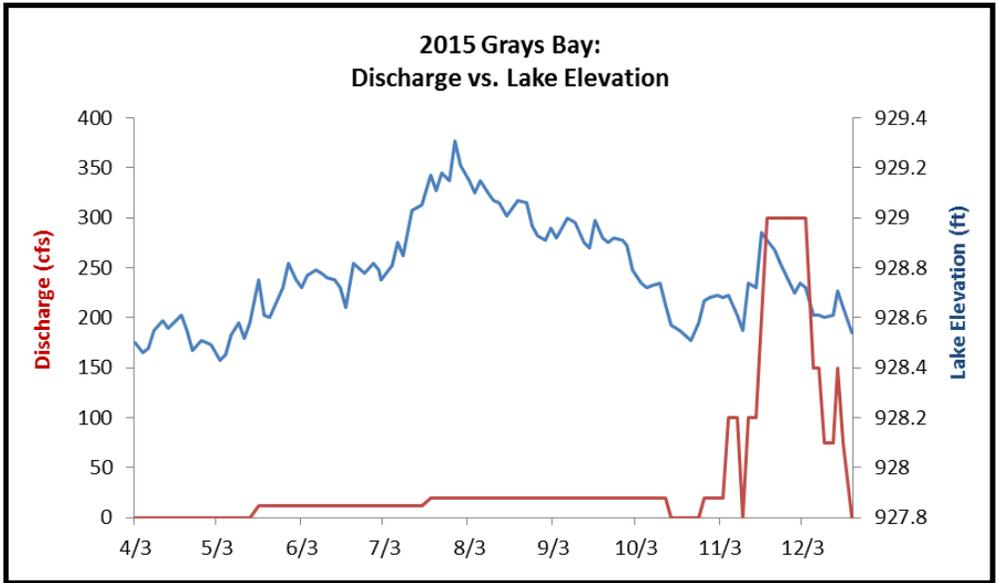
Figure 6. Discharge compared to Lake Minnetonka: Grays Bay Elevation in 2015.
