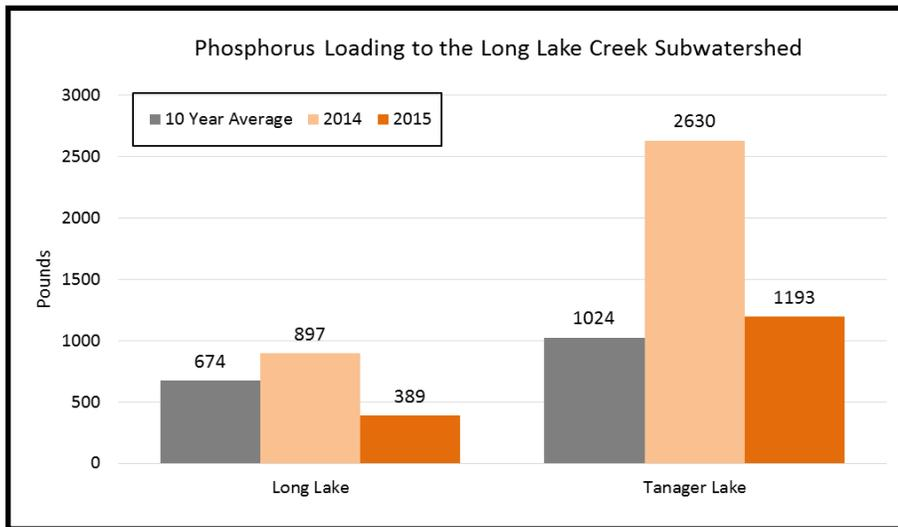
With a watershed to lake area ratio of 151:1, external loading into Tanager Lake is one of the main reasons the lake is impaired for excessive nutrients (Table 19). The other reason is internal loading. Tanager was the receiving waters for high concentrations of phosphorus for a period up to 59 years. The waste-water treatment plant was decommissioned by the late 1980s (MCWD 2007).
