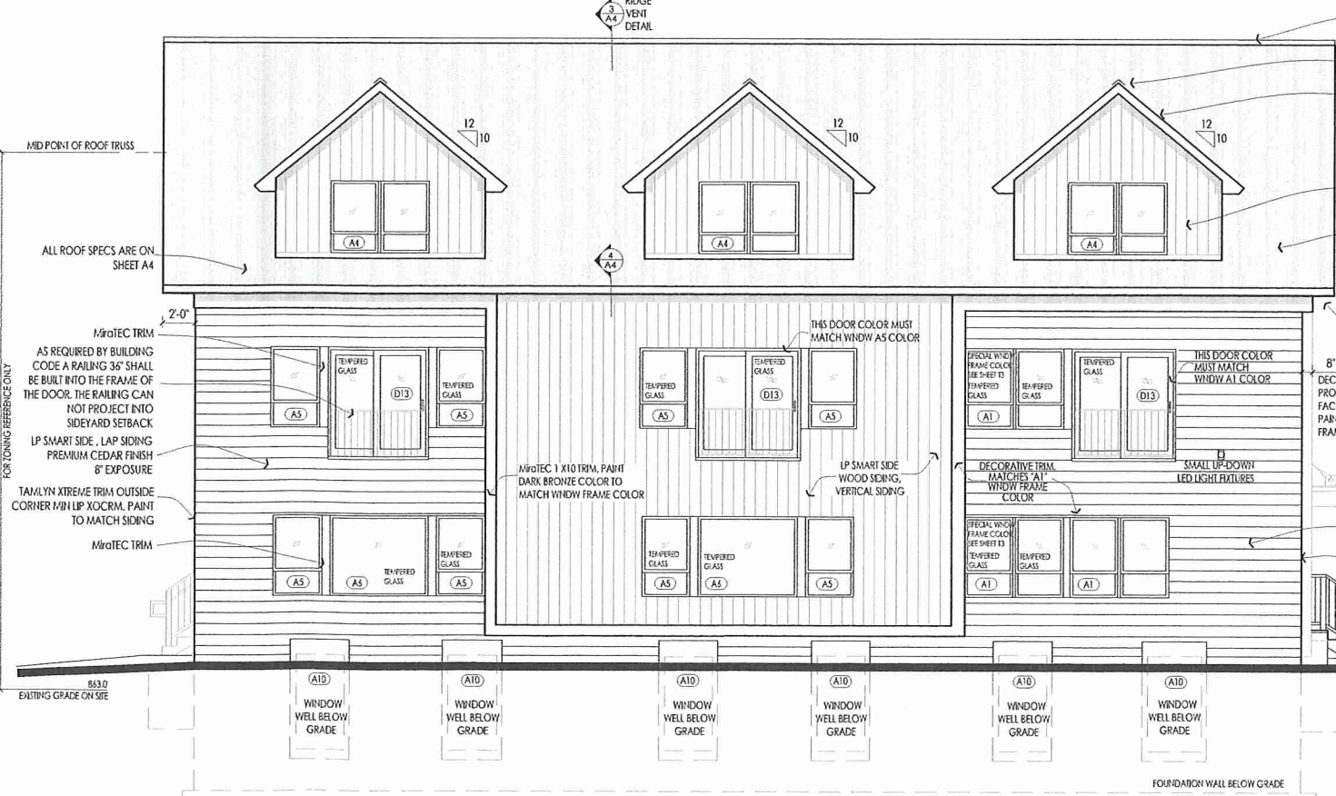
SIDE ELEVATION (NORTH) SCALE: 3/16" = 1'-0"
